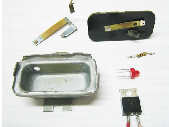
Upper left: the resistance-wire wrapped bimetallic element of an old-fashioned thermal Voltage Stabilizer. Lower right: a solid-state electronic voltage regulator that can be used to replace it.
