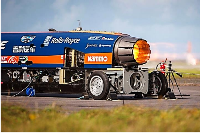
The car's Rolls-Royce EJ200 jet engine is from a Eurofighter Typhoon
