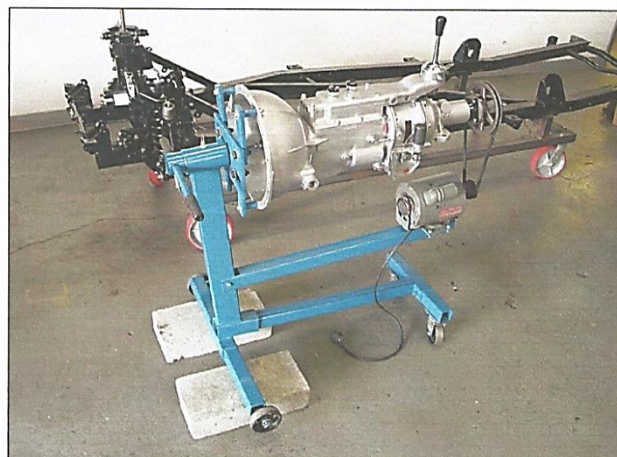
Completed gearbox and overdrive on the Brian Schlorff test stand.
