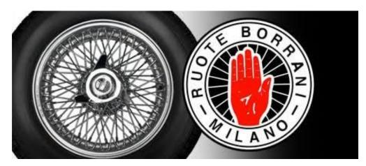
Carlo Borrani was actually born in Calfornia but started up a new company with a partner in Milan using the patented Rudge-Whitworth design of a tapered splined hub to which a tapered wheel's centre could swiftly be fitted and locked into position by means of a single wheel nut or a knockoff. As you know, one uses a suitable hammer to tighten or loosen the knock-off.
